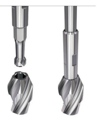
The reamer head can be removed from the flexible shaft with the removal tool. Place the reamer head in the slot on the side of the removal tool. Hold the removal tool with one hand whilst pulling on the flexible shaft with the other. The reamer head will detach from the shaft.
